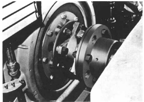
CMR coupling between engine and reciprocating compressor.
